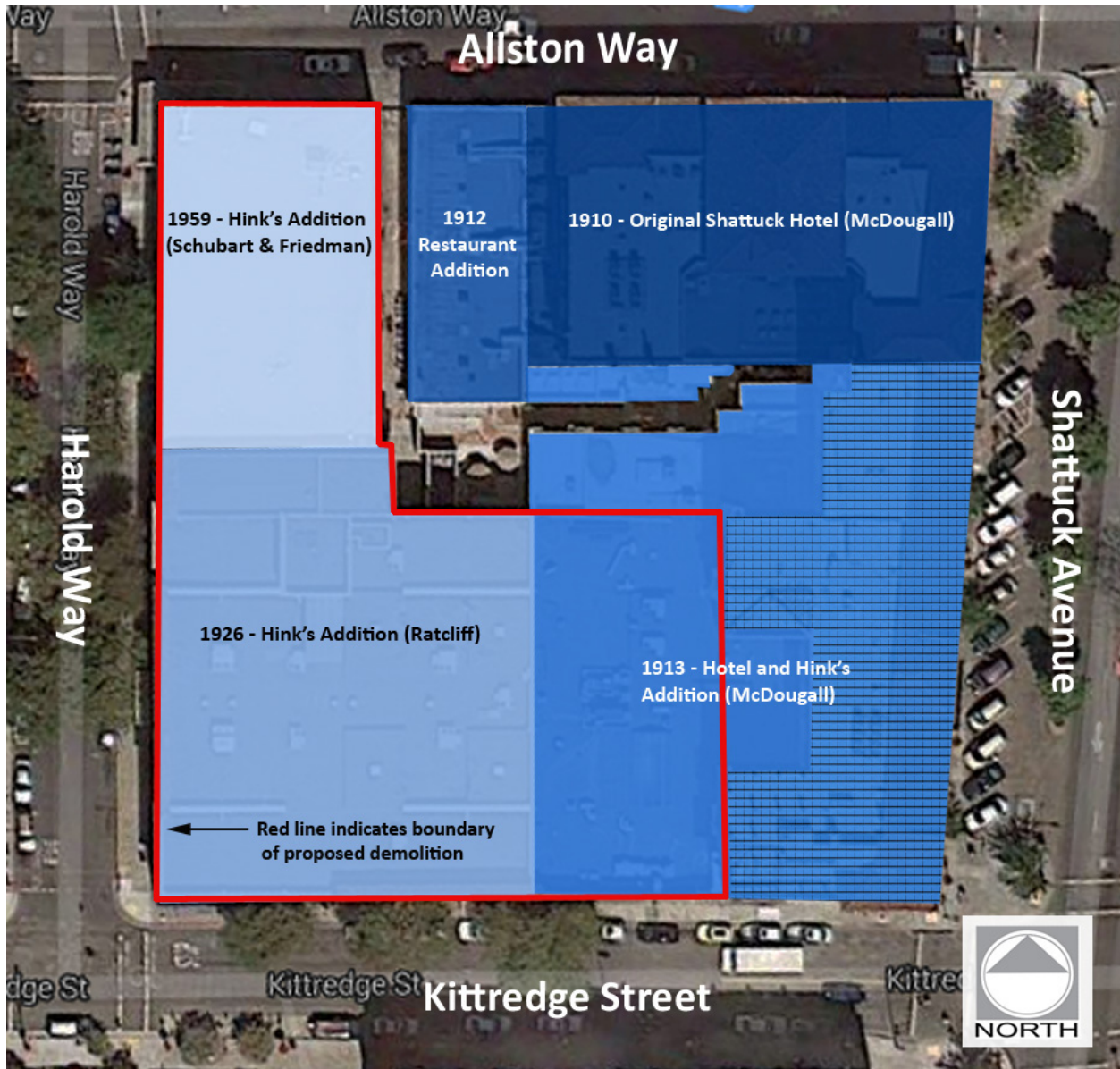
Figure 4-1. Google Aerial view of project block showing construction chronology and area of proposed demolition. The cross-hatched area of the 1913 addition is five stories in height; the remainder of the addition is one story. Note that though the architect of the 1912 addition was likely McDougall, this was not confirmed by archival research. (Google Aerial amended by author, February 2014.)
